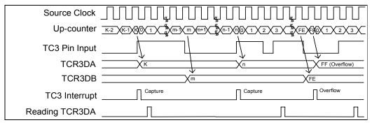
Fig. 5-23 Timing Chart of Capture Mode
